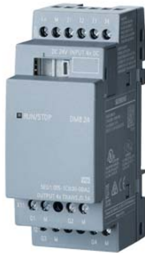
LOGO! DM8 24 EXPANSION MODULE, PU/I/O: 24V/24V/TRANS., 4 DI/4 DO FOR LOGO! 8
