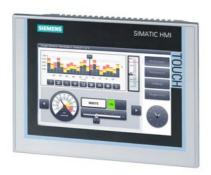
SIMATIC HMI TP700 Comfort, Comfort Panel, touch operation, 7" widescreen TFT display, 16 million colors, PROFINET interface, MPI/PROFIBUS DP interface, 12 MB configuration memory, Windows CE 6.0, configurable from WinCC Comfort
